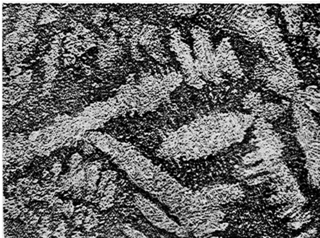
Photo. 2 \times 80 , 34 wt. % \text{KNO}_3 (Medium Cooling)
