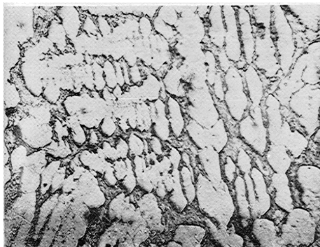
Photo. 5 \times 75 , 82 wt. % \text{KNO}_3 (Slow Cooling)
